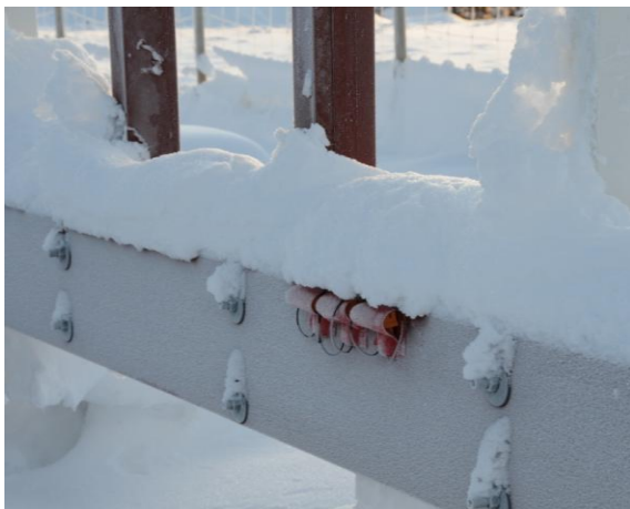
Figure 5. a) A beam with sensors after cold and snowy weather. b) Installation on a façade, sensor behind sheet metal painted in the same color as the wall.
