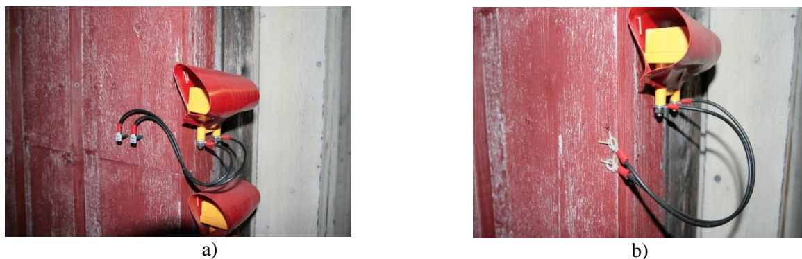
Figure 1. a) HygroTrac sensor nail b) Ring terminals that have been attached to the surface with plastic clamps.
