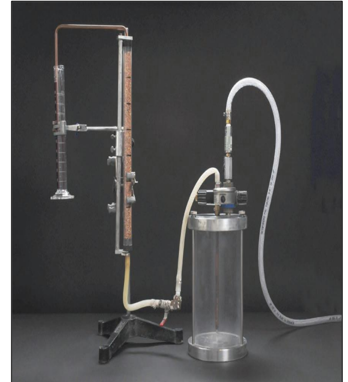
2) Example of a commercially available injectability apparatus with an empty column
